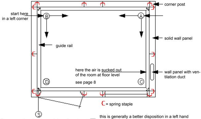
For a room placed against a right wall you have to finish the last corner by loosening the screw marked S and push that end of the wall 2,5 cm outwards to make room for the rubber seals, see page 6. Then push the wall back and replace the screw S.
