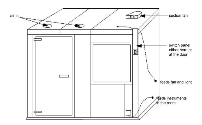
the four conductor cable goes through a hole drilled in the roof to the light fixture, and the three conductor cable to the fan housing (green/yellow is earth)
