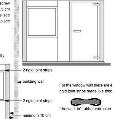
in a right hand corner, this is generally the best way to build the front wall
